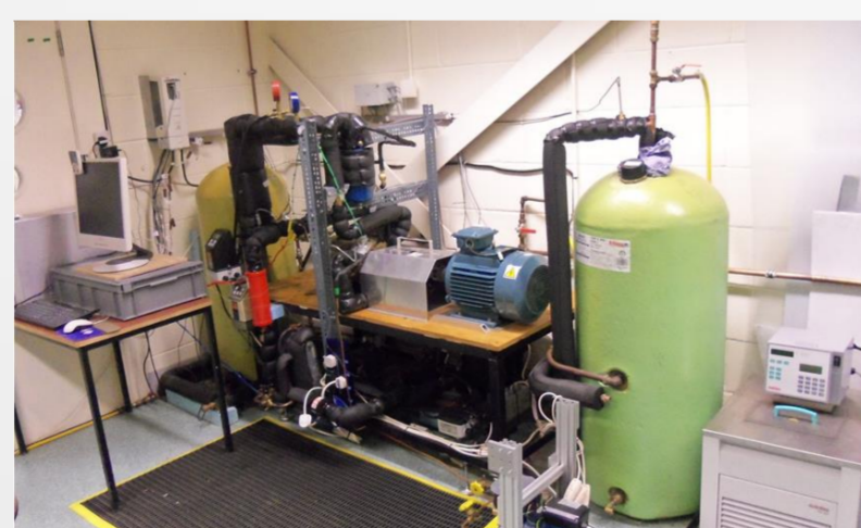
Economised vapour injection and rotary compressor & expander units under development and test
