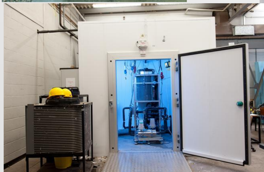
Economised vapour injection and rotary compressor & expander units under development and test
