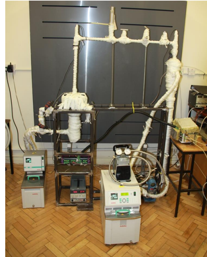
Adsorption test bench for equilibrium property and adsorption capacity
