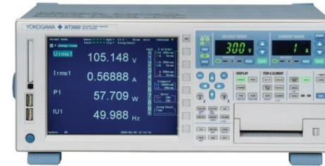
Electricity power meter
